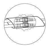
7. Secure one of the anchor points on the side of the arm closest to the light assembly that points to the corner pole where you want the wiring to run out from by removing the backing and pressing the adhesive back firmly for several seconds. Continue to install the remaining anchor points along the arm evenly between the first one and the corner bracket of the Aluminum Pavilion.
