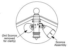
4. Place the piece of shrink tubing over the wires coming out from the side of the center post on the light assembly. Insert both wires into the same end of the shrink tubing.
