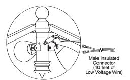
6. Slide the shrink tubing over the insulted connectors and apply heat using a hair dryer, heat gun or other portable heat source. This will cause the tubing to shrink down and fit securely over this connection but still be removable if service is required. DO NOT APPLY OPEN FLAME DIRECTLY TO THE SHRINK TUBING OR THE INSULATED CONNECTORS.
