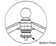
2. This finial can now be screwed onto the bottom of the center post of the light assembly.
