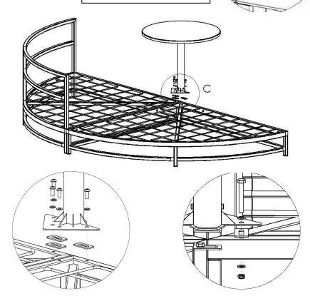
Stainless Steel: Install Pan Head Screws with Lock Washers. Fully tighten with Hex Key (4 places). Aluminum: Install Hex Head Cap Screws with Flat Washers above and Flat Washers with Lock Nuts underneath. Fully tighten with Wrenches (4 places).
