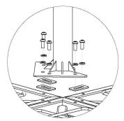
Stainless Steel: Install Socket Head Cap Screws with Lock Washers. Fully tighten with Hex Key (5 places).
