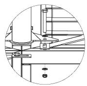
Aluminum: Install Hex Head Screws with Flat Washers above and Flat Washers with Lock Nuts underneath. Fully tighten with Wrenches (8 places).
