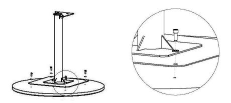
Fully tighten all screws using the Hex Key (4 places).
